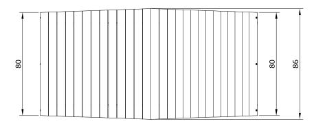
Material frame: steel sheet S235JR 8,0mm and tube S235JRH ø 168x6 mm
