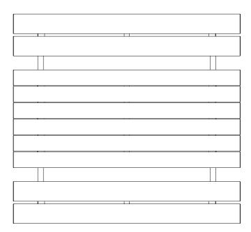
**Material frame**: tubular steel S235JRH, 42,0x2,0 mm **Material seat**: untreated FSC certified Movingui
